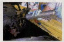
Brent Parry's Challenger took farther to stop from 60 mph than it did when new, so Parry knew his car needed help. He started the MCB upgrade by securing his Mopar on jackstands, disconnecting the battery and pulling off the front tires. Then he used a master-cylinder siphon to drain the brake fluid.
