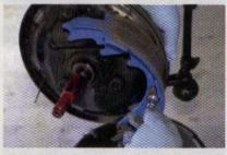
To disassemble the driver-side front brake drum, Parry removed the secondary show spring, the anchor, the primary return spring and the cable guide. Next, the primary shoe retainer, springs and retaining nail came off, followed by the secondary show retainer, spring and nail.
