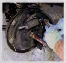
After "dressing" the contact areas on the drum brake backing plate, Parry applied liberal amounts of antiseize compound. Then he installed the new shoe-retaining nails provided in the kit. MCB clearly labels the shoes "primary" and "secondary" to avoid any confusion. The first to go on was the secondary shoe, followed by its retaining spring and retainer, and then the OE brake shoe anchor. Once the secondary shoe was on, Parry installed the Heavier Trick (return) Spring and adjuster cable.
