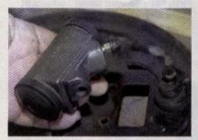
6 After removing and discarding the old Mopar wheel cylinder, Parry installed the MCB high-volume wheel cylinder using the new bolts provided in the kit.
