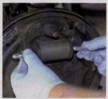
On goes the OE 11-inch Mopar drum brake backing plate, followed by the plungers. Parry used plenty of antiseize compound with the plungers.
