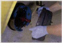
2During initial teardown, Parry checked the condition of all front wheel bearings and front seals, then put them in a plastic bag to reuse later. If you have any doubt about these parts' condition, replace them.
