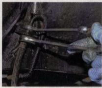
Parry removed the driver-side brake hose from the brake line junction. Then the old hose was removed from the wheel cylinder.
