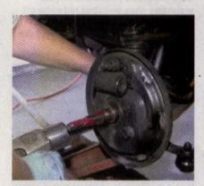
Susing a floor jack to take the tension off the lower control arm, Parry removed the two bolts that secured the lower portion of the backing plate to the lower control arm/ball joint assembly.
