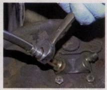
Next, Parry installed the kit's braided stainless brake line, first to the junction at the back of the high-volume wheel cylinder, and then at the hard line junction.
