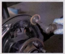
14 Prepping the rear backing plate was a two-step process. First, Parry sprayed liberal amounts of brake cleaner on the plate to get rid of accumulated brake dust. Then he buffed the contact areas on the plate using a small grinder, and followed that step with liberal amounts of antiseize.
