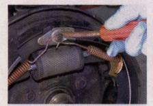
10 The primary brake shoe was next, along with the Heavier Trick Spring and retainer. Parry then installed the star, or adjuster wheel, and brakelever spring. This is all-new hardware provided in the kit. He finished this side by hooking the lever spring to the adjuster lever.
