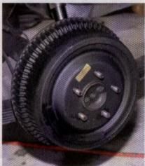
17 The finished driver-side rear brake looked like this after Parry put on the cryogenically treated brake drum.
