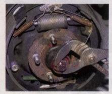
11 Next on the agenda was the installation of the front hub. Parry greased the front wheel bearings, installed a new seal in the front hub and then put the hub on the car. The hub is now technically "free-floating."
