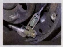
16 Here you can see the completed dadjuster wheel, lever spring and adjuster overload spring assemblies in place. The shoe installation was done.
