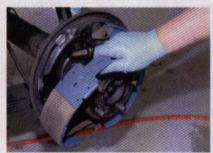
13 The procedure for the rear brakes is similar to that done on the front. Rear drum disassembly began with the removal of the OE secondary return spring, followed by the primary retainer and spring, then the primary brake shoe. Once the primary shoe was off, the secondary shoe and strut rod came off. Parry then moved around to the back side of the backing plate to remove the rear hard line.
