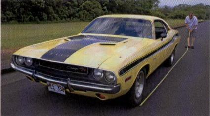
**21** With the system fully installed, Parry conducted a series of three 60-0-mph brake tests, achieving a best stopping distance of 123 feet, a full 49 feet shorter than with the antiquated OE system. As the brakes bed in, that distance will get even shorter.
