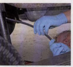
18 The only thing that remained on this side was the installation of the brake line (provided in the kit) from the junction to the crossover hard line. Then Parry repeated these steps for the passenger-side rear brake.
